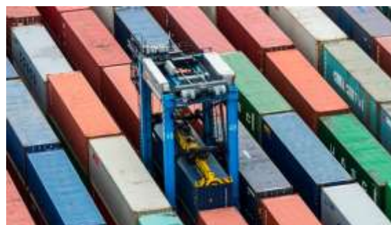
Figure No 6. Straddle Carrier storing a container Source: (CROZEL, 2019)
