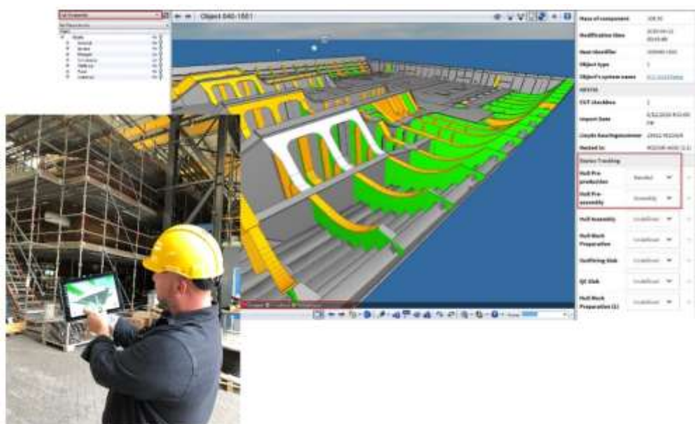
Fig.4: Example of using a 3D model in the CADMATIC eShare platform at a production site.
